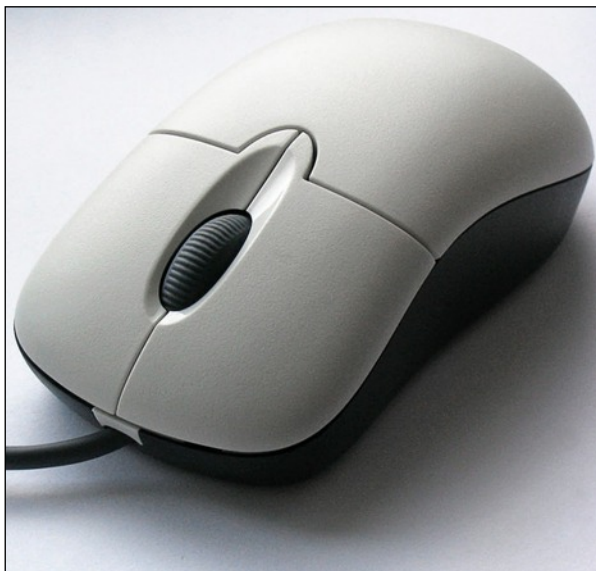
Fig. 2. A standard “wired” mouse comes with two “click buttons” (left and right), and a central scroll wheel.
