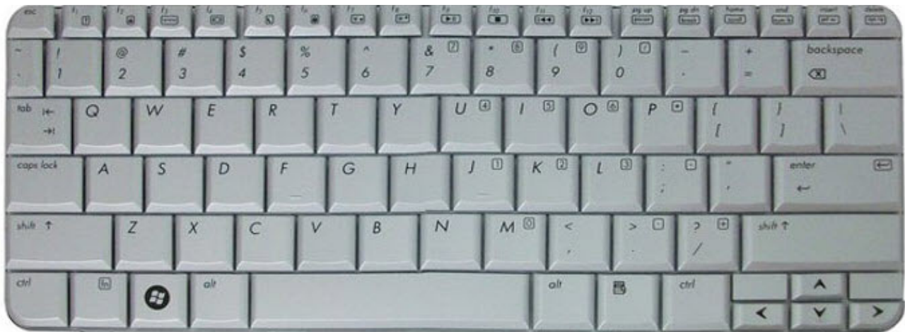
Fig. 1. A typical laptop keyboard layout differs from a typewriter keyboard in that it has 12 “function” keys along the top row, and “escape” key at top-left, Control (Ctrl) and Alternate (Alt) keys to the left and right of the space bar, and four “Arrow” keys for moving the cursor around on the screen.
